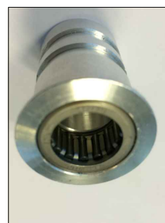
Top bracket Drill diameter 25 mm
