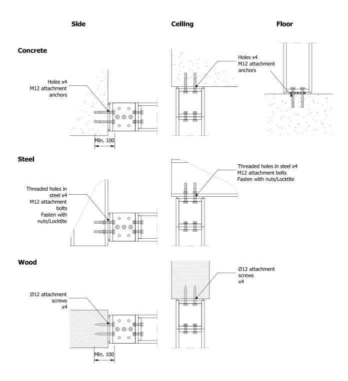
Drill if necessary to increase threaded M12 holes in cubes (to  $\emptyset$ 13mm) Use washers, hex head bolts and screws Close joints with sealant
